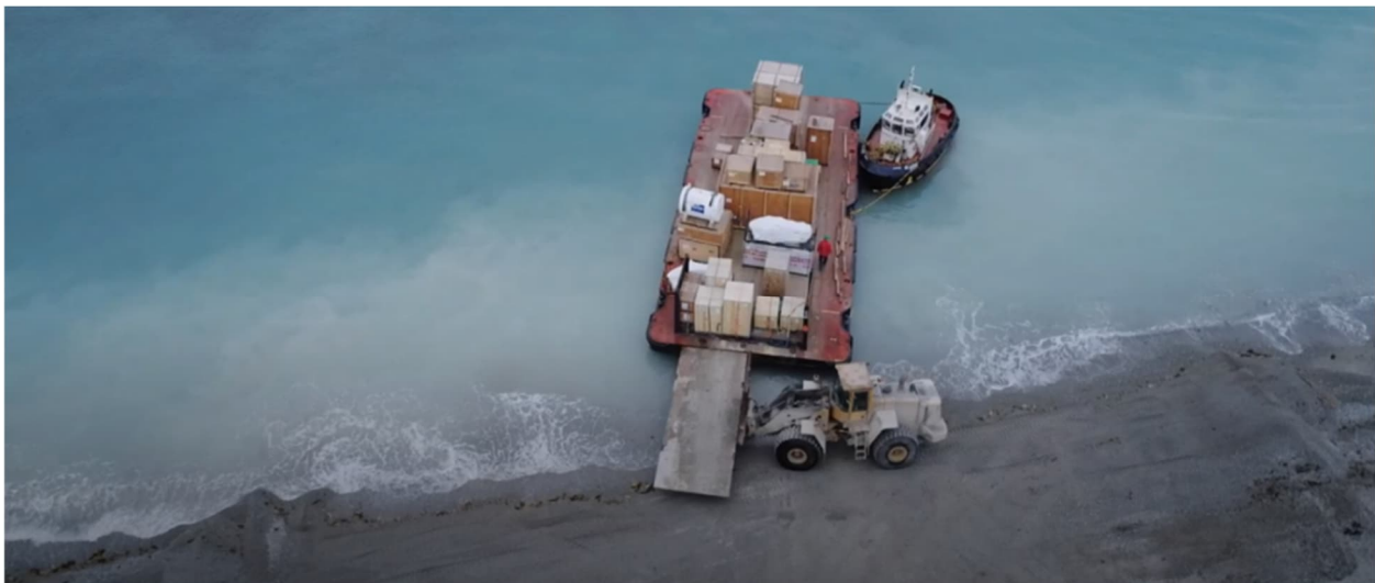
Figure 2-2 Sealift barge with tug at beach with loader installing ramp (courtesy of CBC's High Arctic Haulers series)
