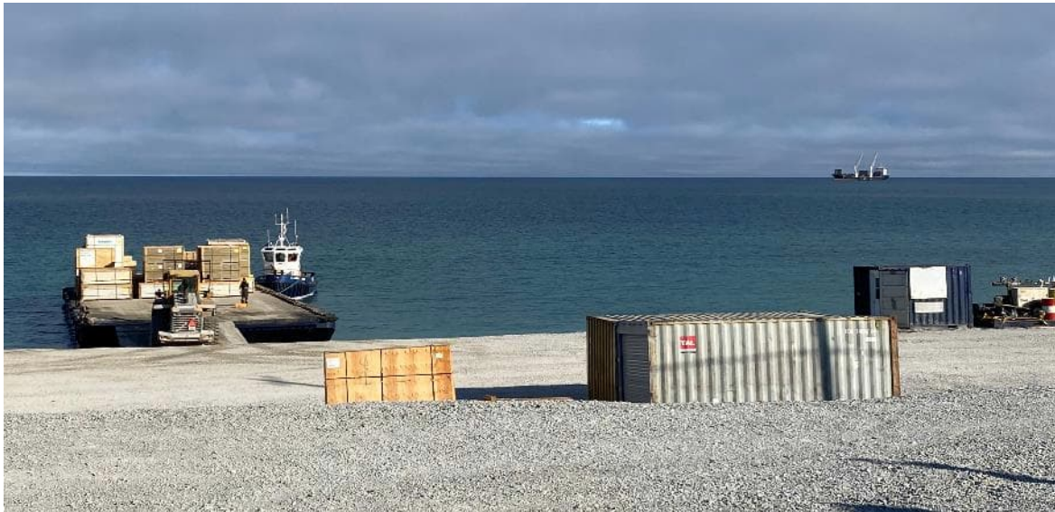
Figure 2-7 Barge lightering operations at Sanirajak sealift beach (2021). Supply ship is shown anchored in the background.
