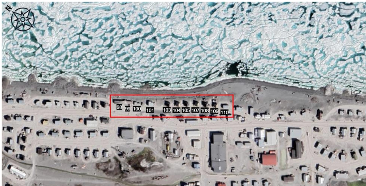
Figure 2-17 High risk houses #98 to #110 threatened by shoreline erosion (Google Earth)
