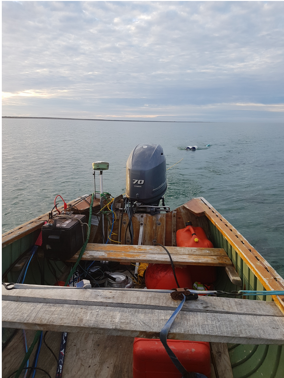
Surveying with towed sub-bottom acoustic profiler
