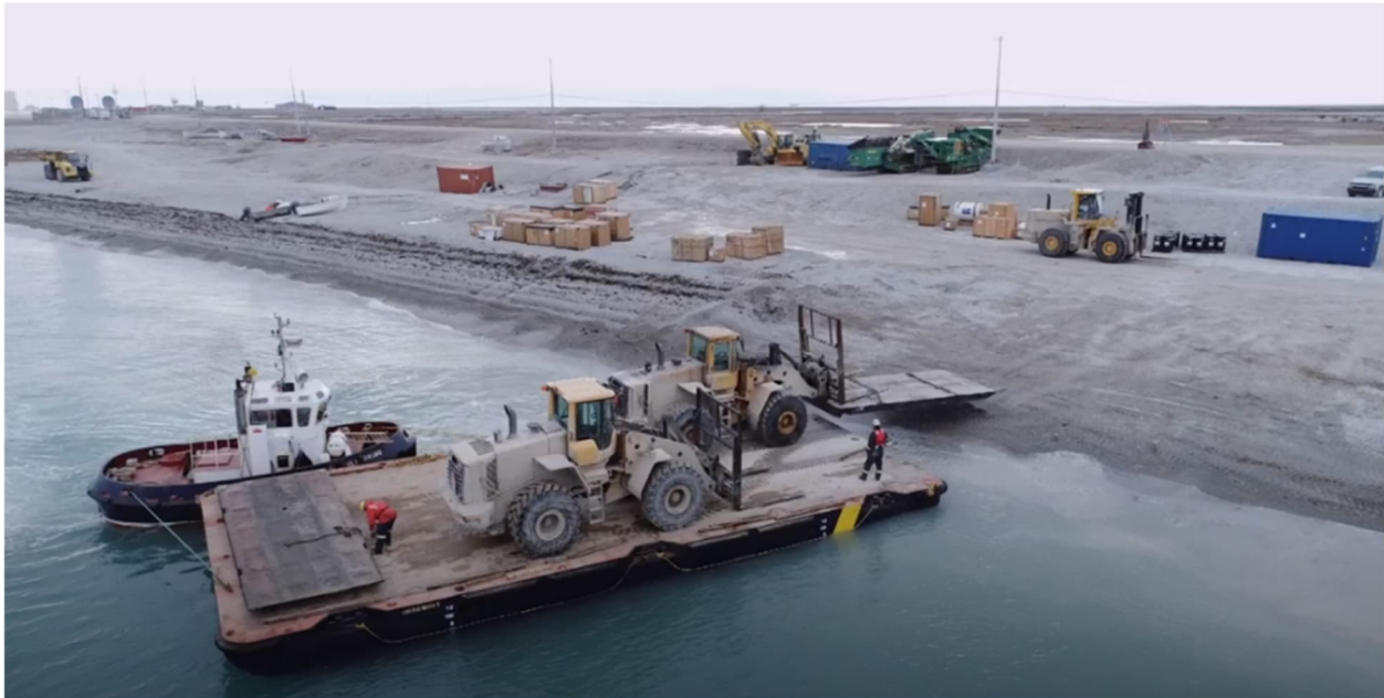
Figure 2-3 Front end loaders removing ramp after unloading operations, tank farm in background (courtesy of CBC's High Arctic Haulers series)
