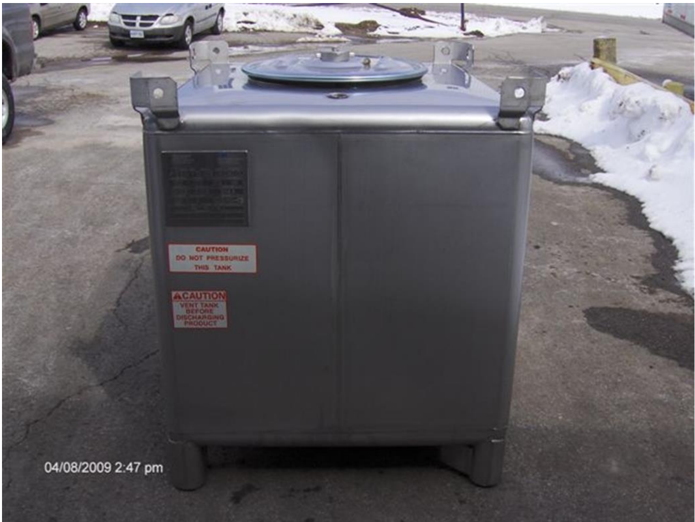
Figure 6: One of the 1,325-litre stainless-steel potable water storage tanks purchased by CGS.
